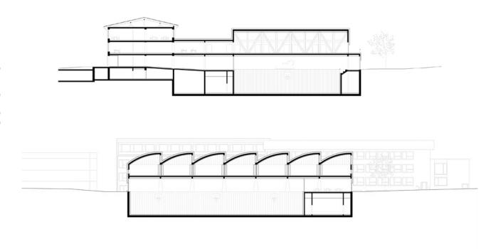
"Light on heavy: The elegant carrying structure – above with columns, below without – creates generous spaces and minimizes excavation work."
